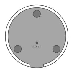
If, for any reason, you must perform a factory reset you need to press the pinhole button for between 10-15 seconds. By pushing the button, all your account settings will be lost and the Hub MINI will return to default.
