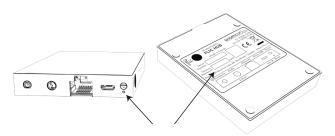
If, for any reason, you must perform a factory reset you need to press the pinhole button for between 10–15 seconds.
