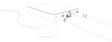
Connect your Flic IR accessory to the Hub via the 2.5mm connector and place the IR blaster in general the direction of the recieving device(s).
